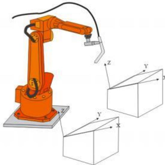
Figure 2.4 Robot user coordinate system
