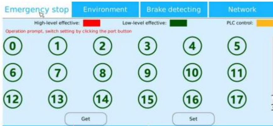
Figure 8.4 Emergency stop output configuration
