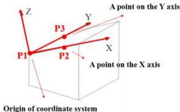
Figure 2.11 Three-point method to establish user coordinate system
