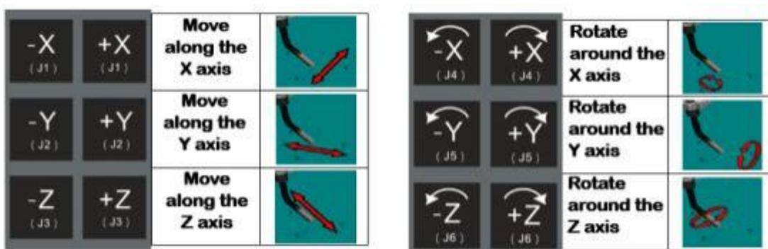
Figure 3.6 Keys function when the operation type is " tool coordinate system"
