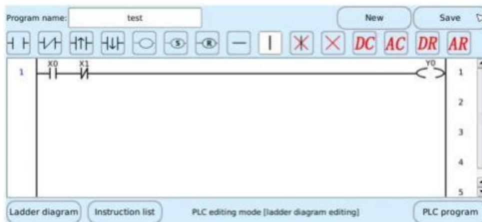
Figure 6.1 PLC programming ladder diagram
