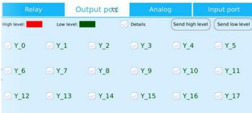
Figure 7.4 Basic port operation interface
