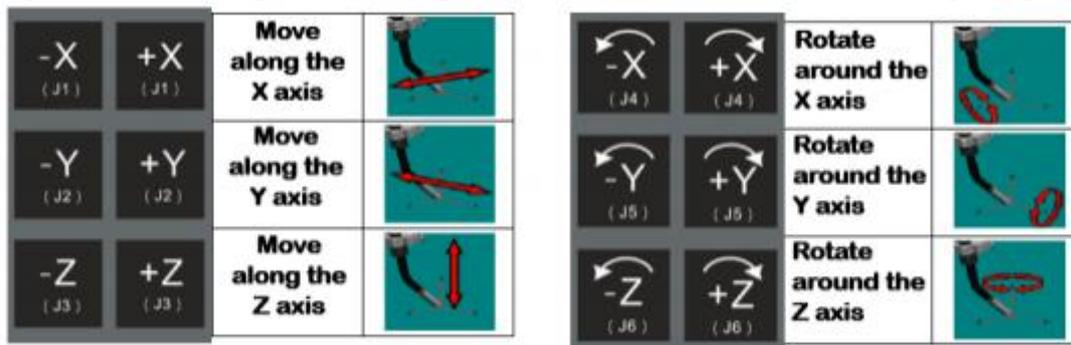
Figure 3.5 Keys function when the operation type is " user coordinate system"
