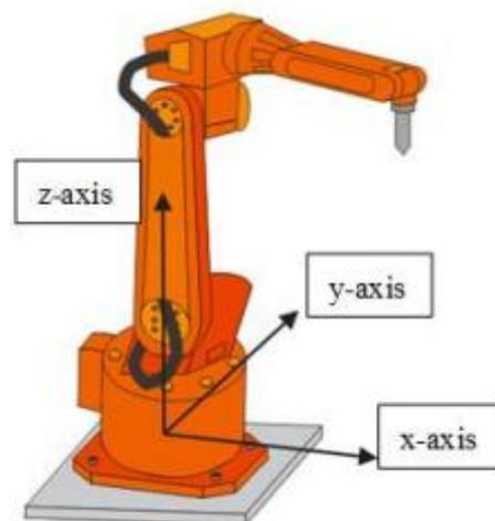
Figure 2.1 Robot base coordinate system
