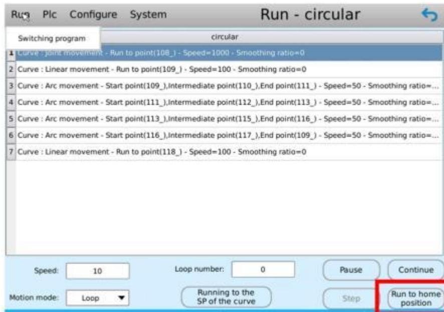
Figure 4.5 "run to home position" button in "automatic mode"
