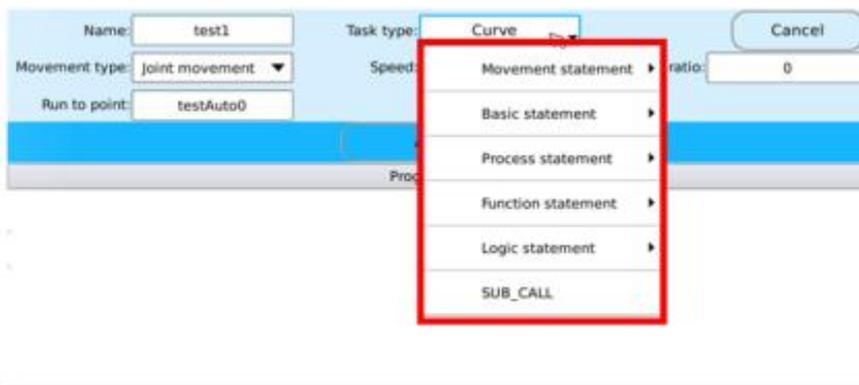
Figure 5.1 Instructions provided in SZGH Robot control system
