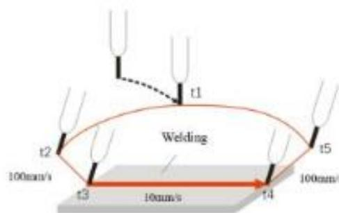
Figure 4.6 Robot motion trajectory for welding
