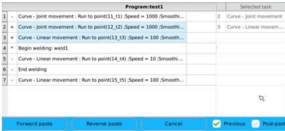
Figure 5.6 Forward or reverse pasting instructions at the specified position
