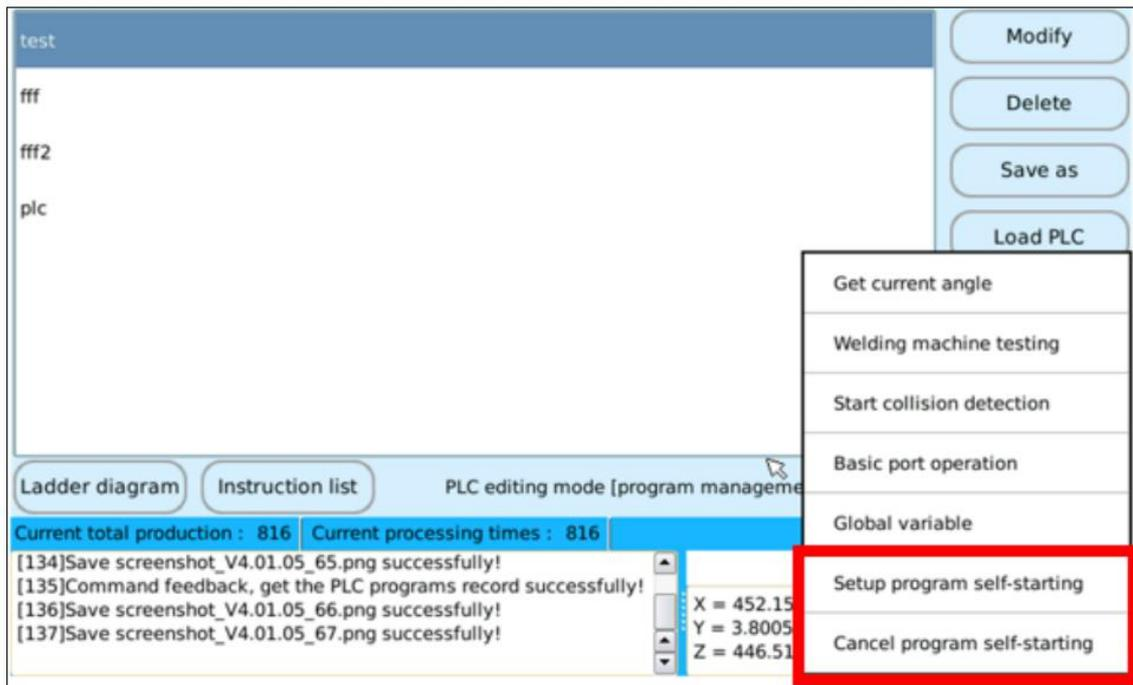
Figure 6.4 Setting the automatic operation of PLC program
