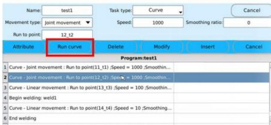
Figure 5.7 [Run curve] button will appear when selecting curve command
