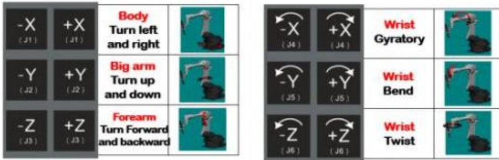
Figure 3.3 Keys function when the operation type is " joint coordinate system"
