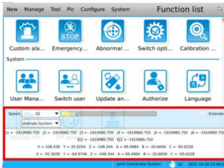
Figure 3.2 Manual teaching configuration and motion monitoring page
