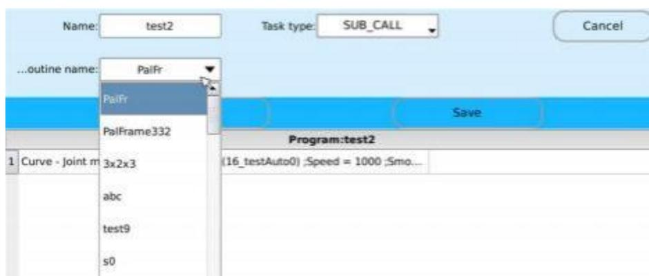
Figure 5.15 Using SUB\_CALL in basic program
