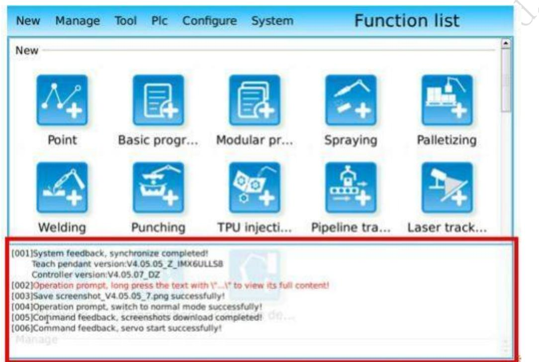
Figure 3.8 Operation feedback display box
