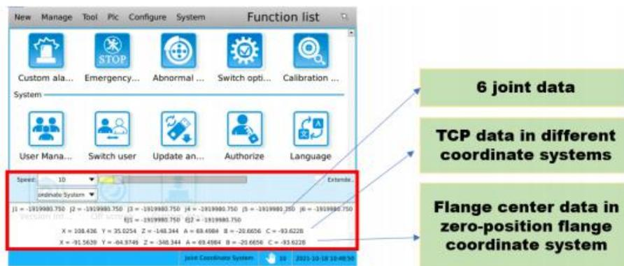
Figure 4.3 Real time display of current "point" information
