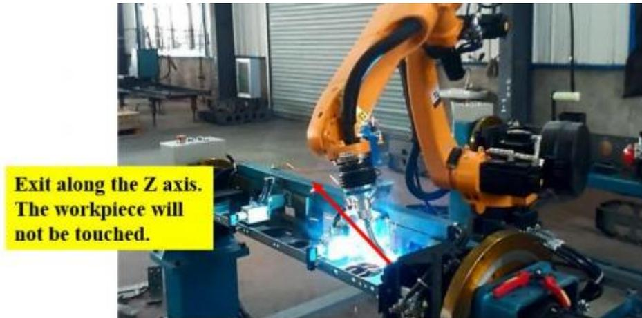
Figure 3.7 Manual teaching in tool coordinate system
