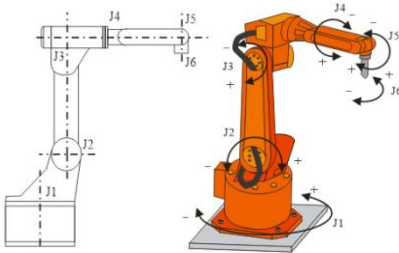
Figure 2.2 Robot joint coordinate system
