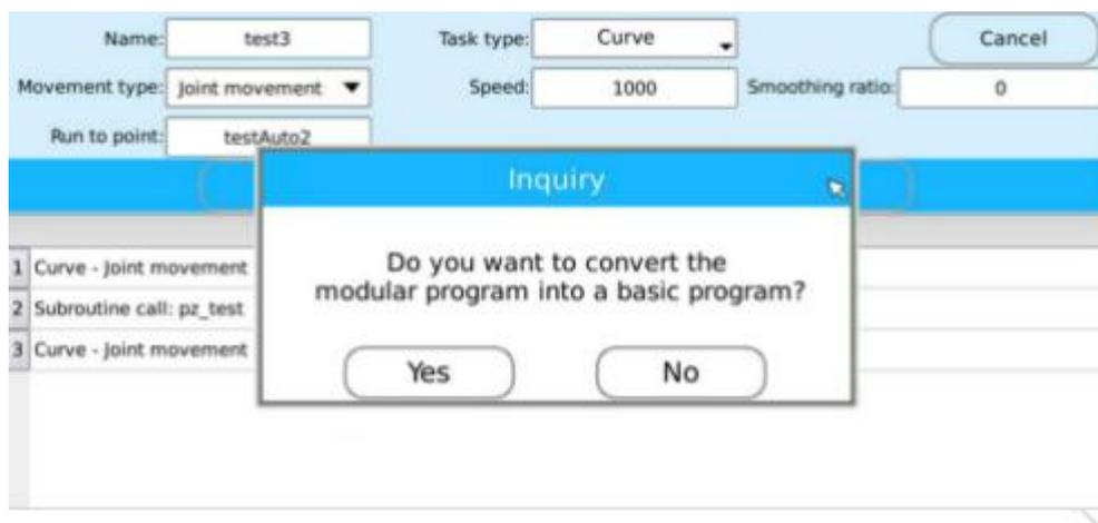
Figure 5.17 "PCALL" task type and usage
