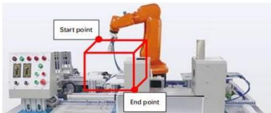
Figure 1.7 Start point and end point of safety zone
