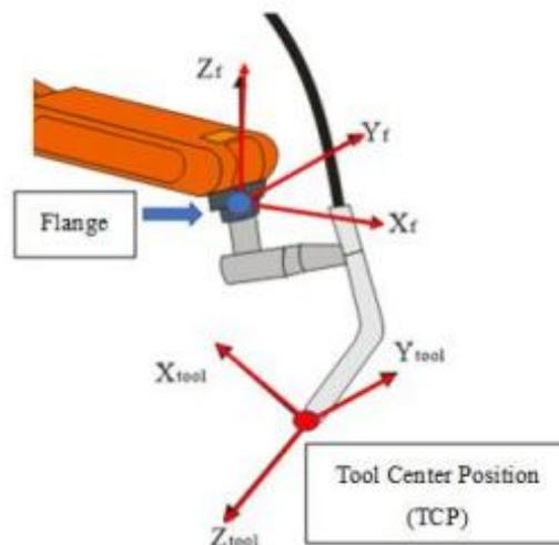
Figure 2.3 Robot tool coordinate system
