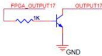
Figure 7.2 Open collector output circuit
