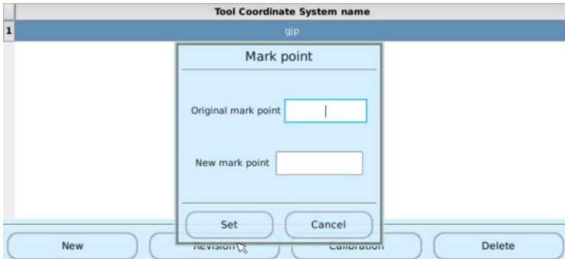
Figure 2.10 Using mark point for rapid calibration
